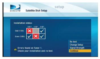
Errors may be displayed on the screen. It is normal to see one or two boxes with an X instead of a ✓. Select Continue.
