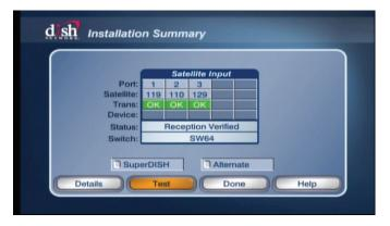
When you see the SW64 as the installed switch, the antenna is ready for use.
