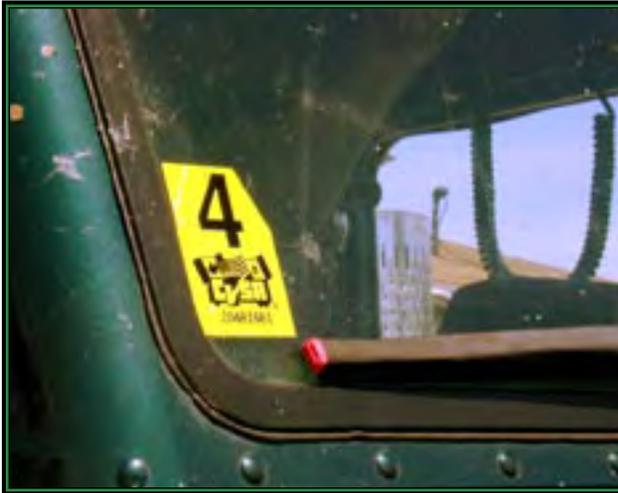
CVSA stickers are color-coded. Based on the color, the year, and the corner removed, officers can determine when a Level 1 inspection was conducted on a given vehicle. Vehicles displaying current CVSA stickers generally are not re-inspected unless there is an obvious driver violation or a noticeable defect in the vehicle or its cargo.
