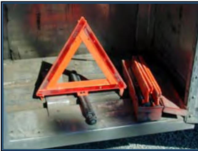
You have a choice of three reflective triangles (left) or liquid-burning flares. Because flares have a limited life, most carriers elect to use emergency reflective triangles; but if you choose flares you must equip each vehicle with enough to last for the most time-consuming breakdown imaginable. Flares may not be used if the materials in transport are explosive, combustible, or flammable.
