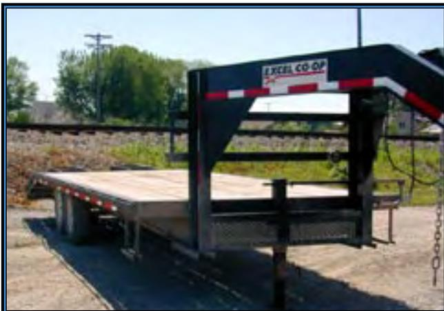
pounds and widths of 80 inches or more must be marked with retroreflective tape. The tape must cover at least 50 percent of the length of each side of the trailer and be evenly distributed across the length.
