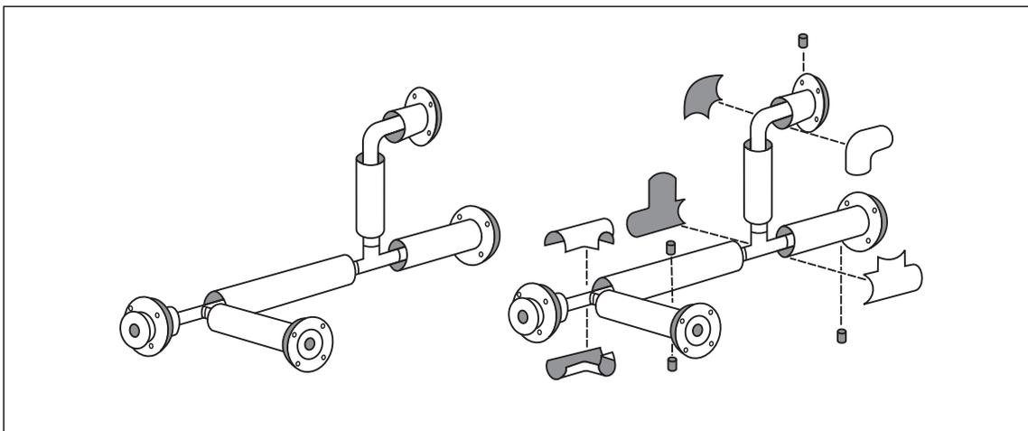
Fig. C.1.3-1. Prefabricated jacketed section
