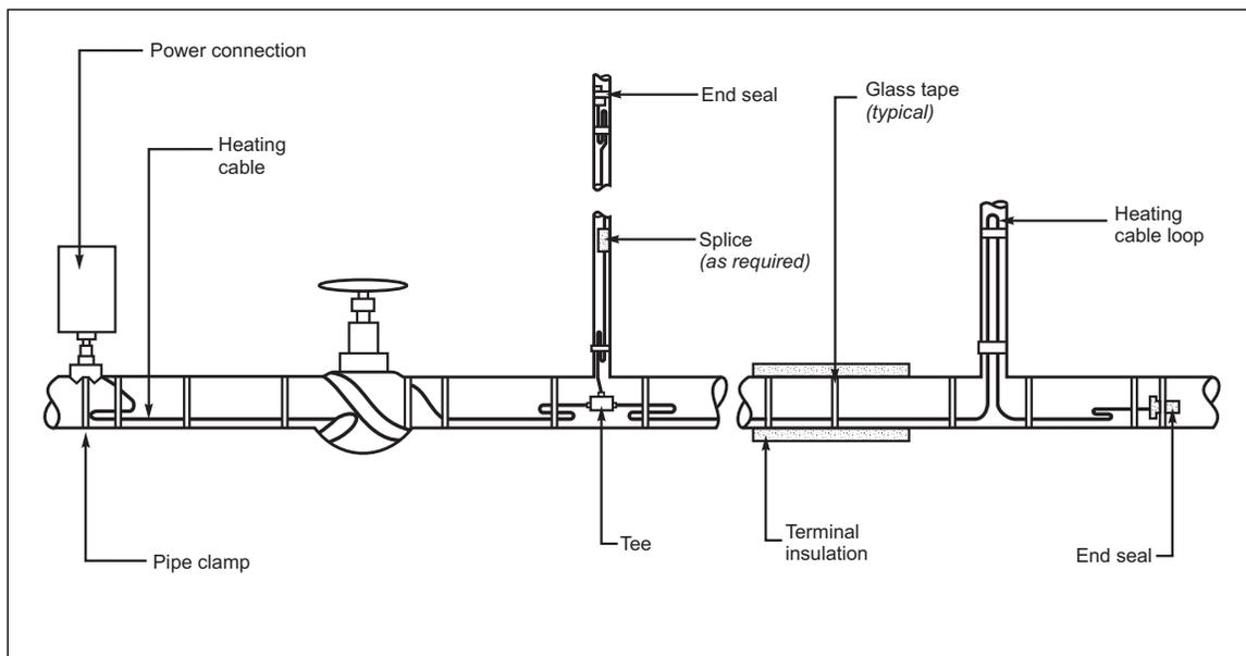
Fig. C.1.1-1. Typical heat tracing system
