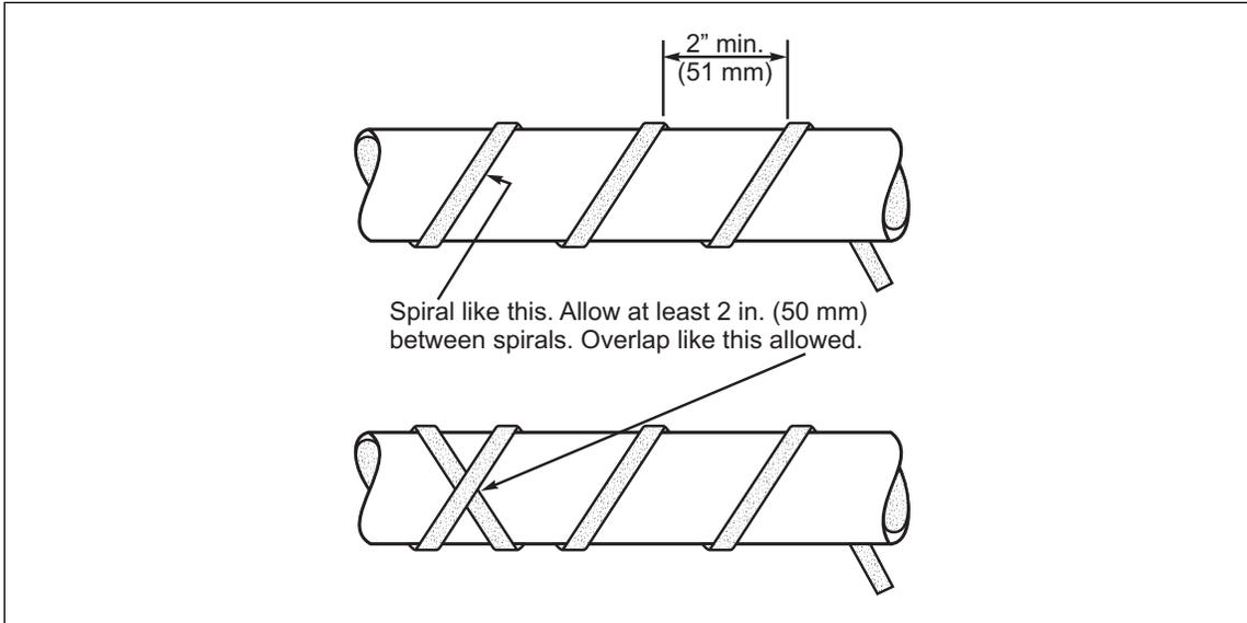
Fig. C.1.2-1. Installation of self-regulating heating cable
