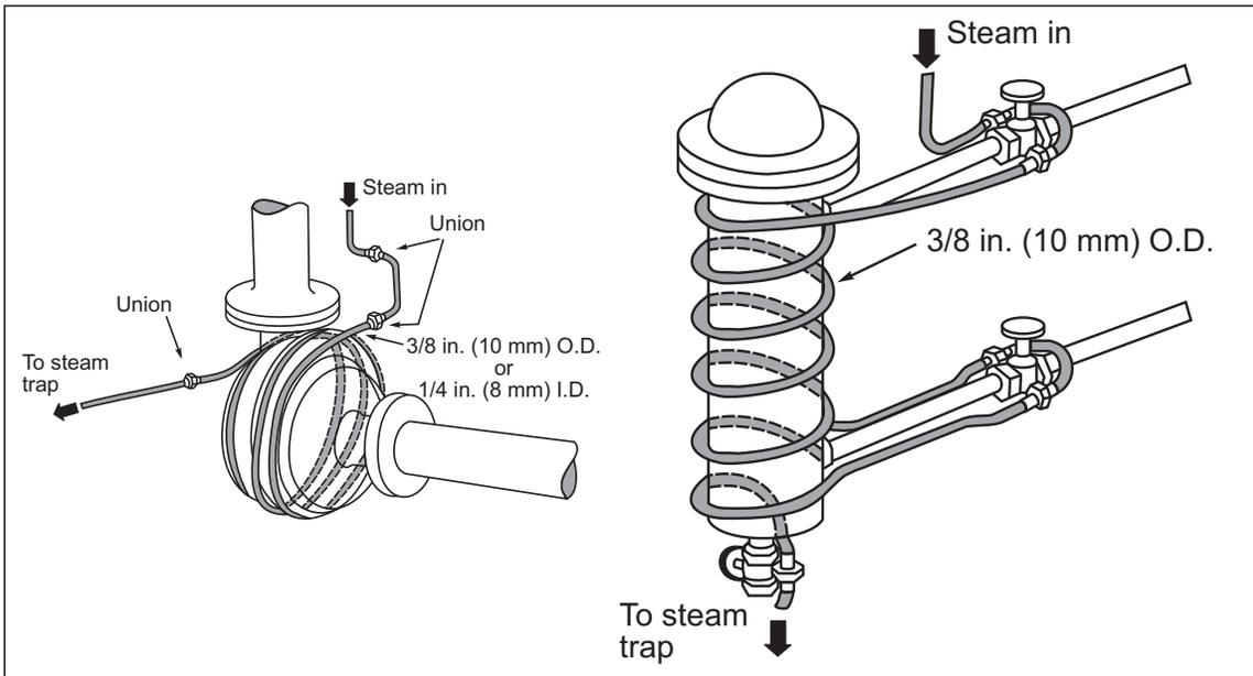
Fig. C.1.5-2. Steam tracer lines around pump casing and typical instrument tracing
