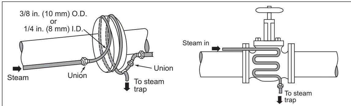
Fig. C.1.5-1. Steam tracer on a flange, on a straight pipe and a valve
